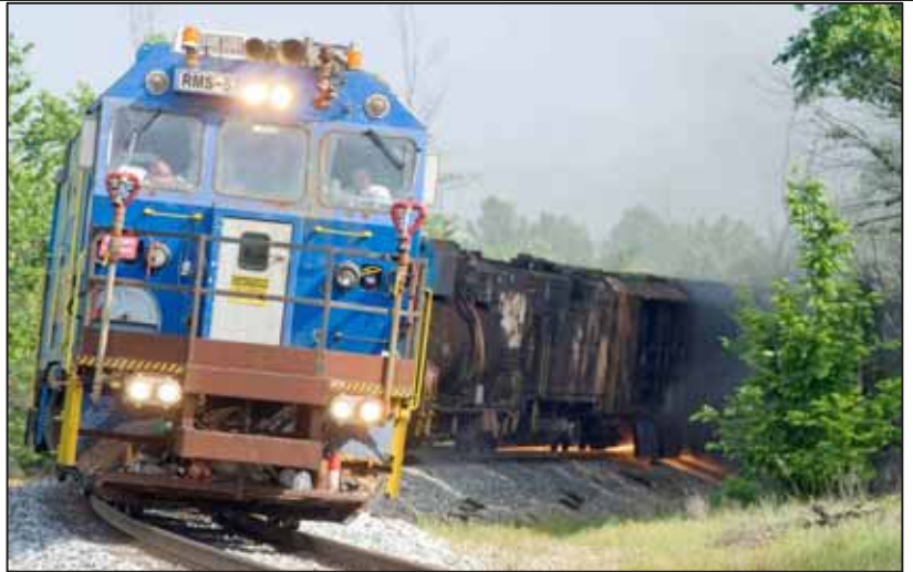
A Pandrol Jackson Railgrinder RMS-5 works its way south through the curve approaching the haul road outside of Earlington Wednesday morning May 28, 2008 on CSX's Henderson Subdivision as it works between Madisonville's Trident and Mortons Junction. According the crew CSX tries to resurface the rails twice a year to improve performance and life of the rail. (Photo by Jim Pearson)
